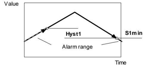
Example of hysteresis setting: S1 as max. switching point and as min. switching point) :
