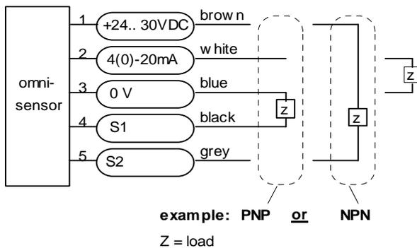
The switchpoints are changing to PNP or NPN depending to your Bitte benutzen interface automatically. Please you use shielded cable, signal lines < 30m and power supply lines < 10m.
