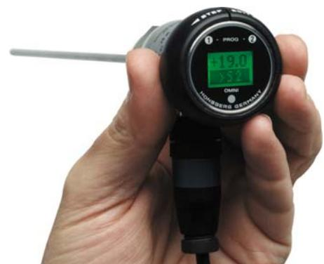
The programming ring can be swivelled to Pos. ① and Pos. ②. The following are actions possible:
